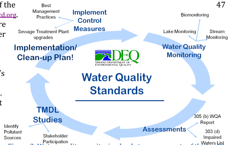
Figure 2. Water quality monitoring leads to assessments of the health of the state's waters. When waters are impaired, a TMDL study is ordered. Once the study identifies pollution sources and creates a "pollution diet" plan, control measures are implemented. Continued monitoring shows whether the control measures are effective. Image: VA DEQ.
